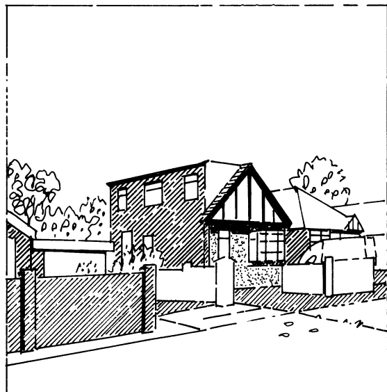
Fig. 9.4 Inappropriate Roof Extension
