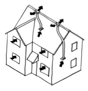
Fig 8 - Passive Stack Ventilation replaces the need for energy hungry extract fans.
